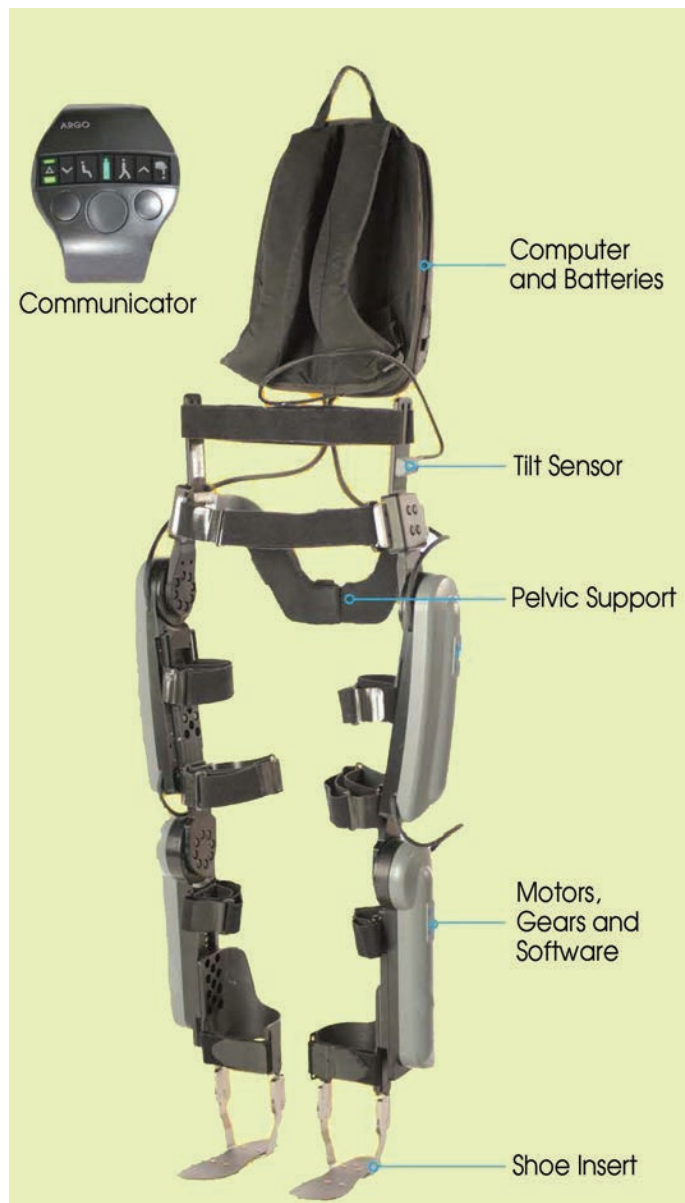
Figure 1. Components of Argo’s ReWalk system. Image courtesy of Argo Medical Technologies.
