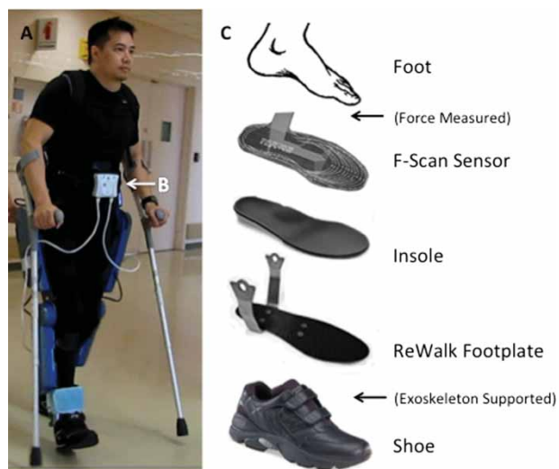
Figure 1 Using F-Scan™ Sensors with the ReWalk™. (A) Participant using the ReWalk™ exoskeletal device; (B) participant wearing F-Scan™ incorporated into the ReWalk™ setup; and (C) F-Scan™ in-shoe pressure sensors placed above the insole below the surface of the foot. The footplate of the ReWalk™ powered exoskeleton sits below the insole of the shoe; the weight of the ReWalk™ is not transferred onto the force sensor. Note: The heel strike as the participant takes a step in the ReWalk™.
